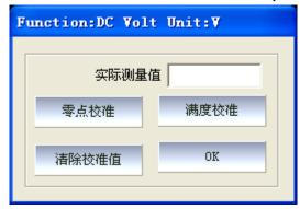
Special Note: the AC signal only need to do full-scale calibration.
